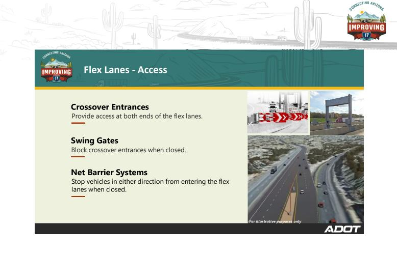
The flex lanes will be equipped with an electronic gate system and net barriers that <u>slow and stop vehicles</u> from entering the roadway in the wrong direction.
