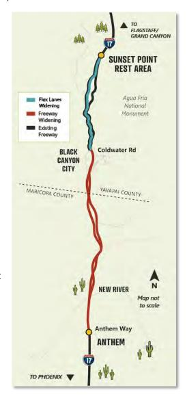
Improving the stretch of I-17 between Anthem Way and Sunset Point includes widening 15 miles of roadway, replacing two bridges and widening 10 others, and constructing approximately 8 miles of flex lanes. The project is located within ADOT's Central and Northwest Districts in Maricopa and Yavapai counties, respectively.
